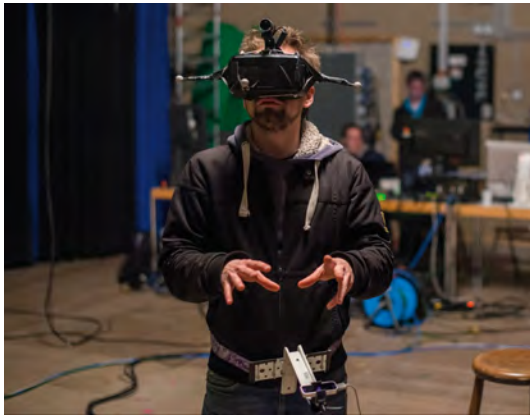
Figure 5: The first prototype combining augmented reality and gesture control for set editing
