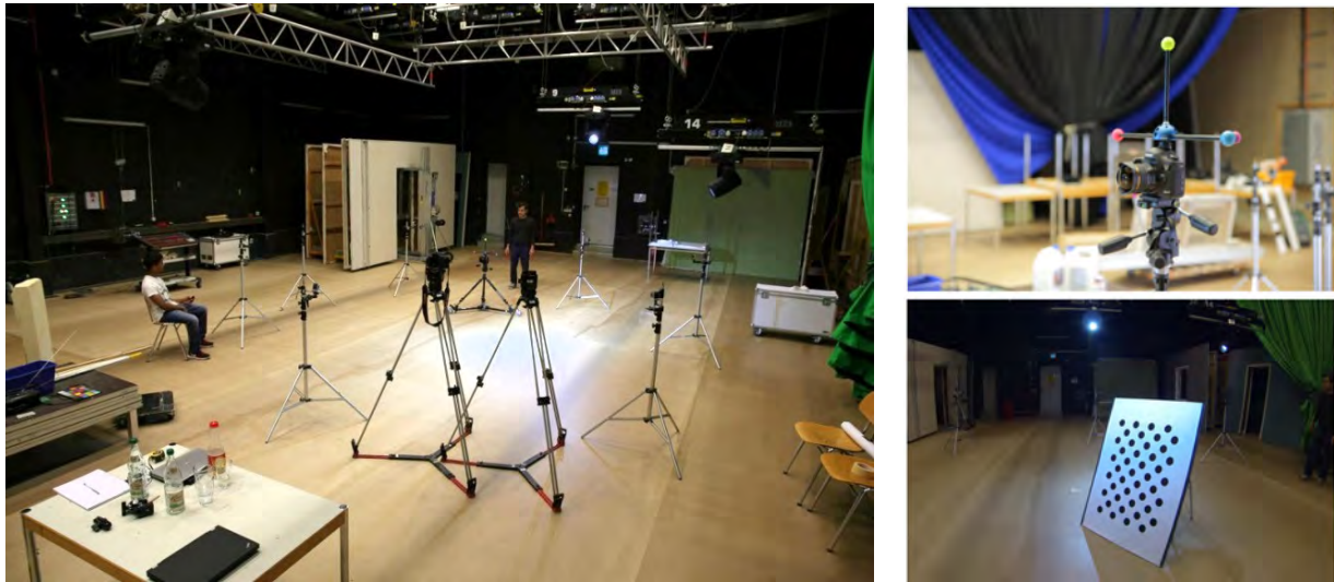
Figure 9: left: Multi-camera setup in the studio incl. the fisheye probing camera on a tripod dolly, bottom-right: Calibration pattern used for registering the witness cameras, top-right: Attached calibration rig for registering the probing camera
