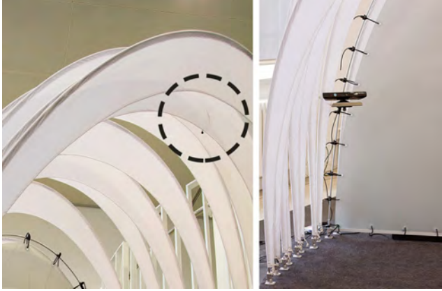
Figure 3: Location of the clip (left) and Kinect (right) microphones (Installation details).
