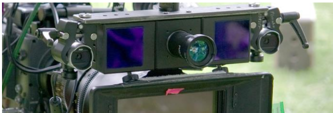
Fig.1: Custom camera rig mounted on an Arri-Alexa
